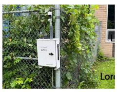
The monitor is an Aeroqual AQS1 unit which measures PM 2.5 (fine particulate matter), NO2 (Nitrogen Dioxide), and O3 (Ozone).
