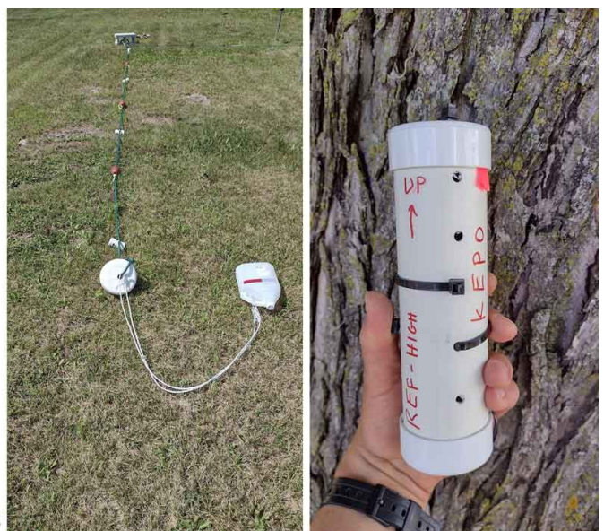
Diagram of “deep” temperature/depth recording station. The top buoy will be removed before lakes freeze. (Left) - Temperature/depth recording station assembled on land. (Center) - Atmospheric pressure sensor to be deployed near Fire Road. (Right)
