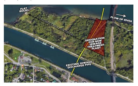
New standards for treatment plants require distances of at least 500 feet from residences. That distance cannot be met on the present site. The current discharge pipe (after treatment) that goes under the seaway and resurfaces on the north side of the seaway would be used for the new plant.
